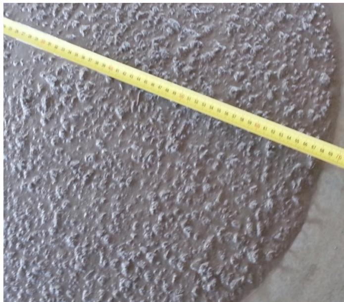
**Figure 3.** Focus on the end of the SCC in the slump flow trial.
