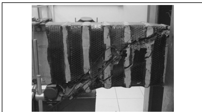
Figure 5 - Detail of failure mode in beams V12_A, V18_A e V20_A.
