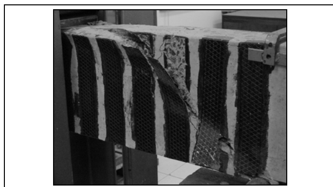
Figure 4 - Detail of failure mode in beams V9_A, V9_B e V21_A.
