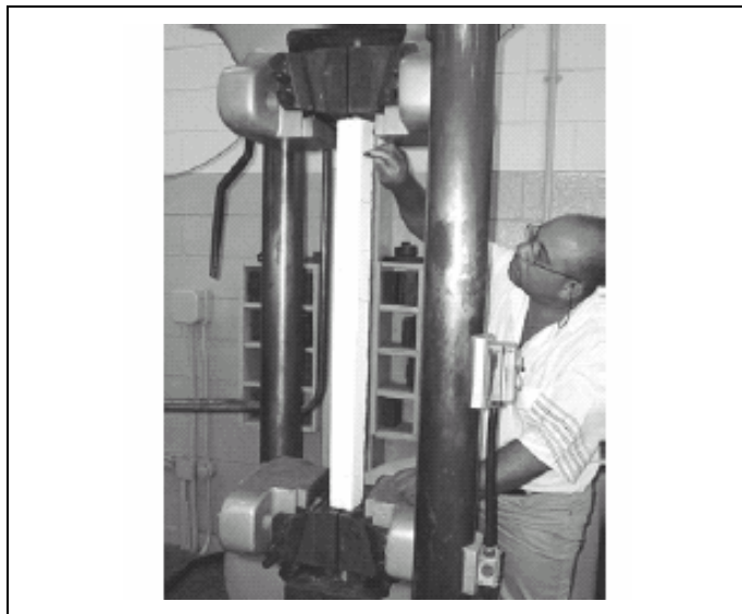
Figure 2 - Loading system and marking of cracks.
