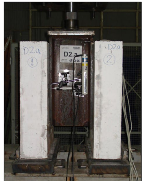
Figure 6. Dimensions of specimens (in mm) and experiment setup (group D2).
