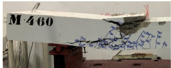
d) Cracks of beam M-460 and beam after the test
