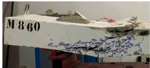
e) Cracks of beam M-860 and beam after the test
