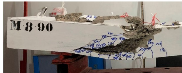
c) Cracks of beam M-890 and beam after the test
