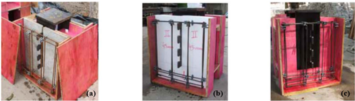
Figure 5. Specimens tested: (a) concrete pre-slab; (b) EPS plate and (c) no pre-slab.
