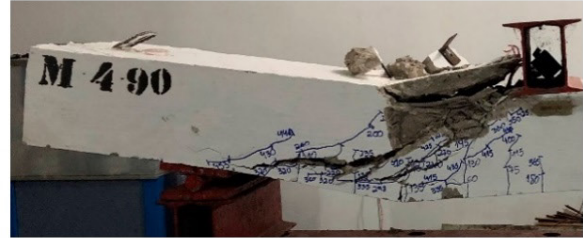
b) Cracks of beam M-490 and beam after the test
