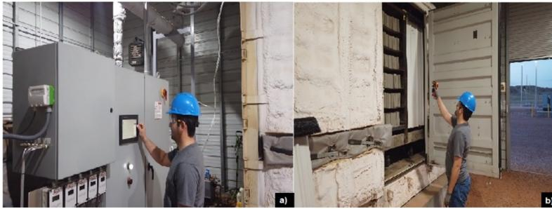
Figure 10. Chamber control: a) CO<sub>2</sub> injection configuration, b) temperature measurement. Source: [[38]].
