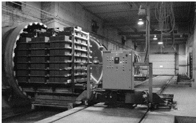
**Figure 7.** Carbonation chamber developed by Carboclave. Source: [[35]].
