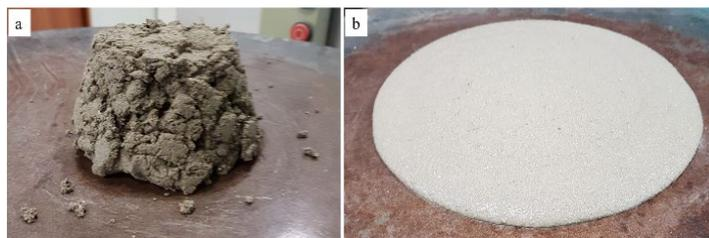
Figure 3. Spread Diameter HEMC – 10% (a), pAve – 10% (b).
