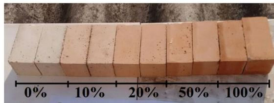
Figure 5. Samples of mortars exposed to atmospheric conditions, aged 28 days.
