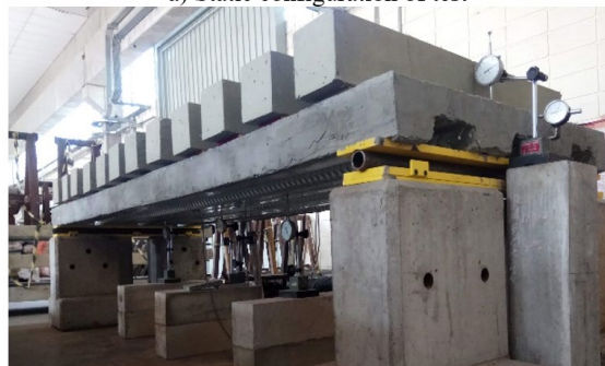
b) Composite slab under service loading
