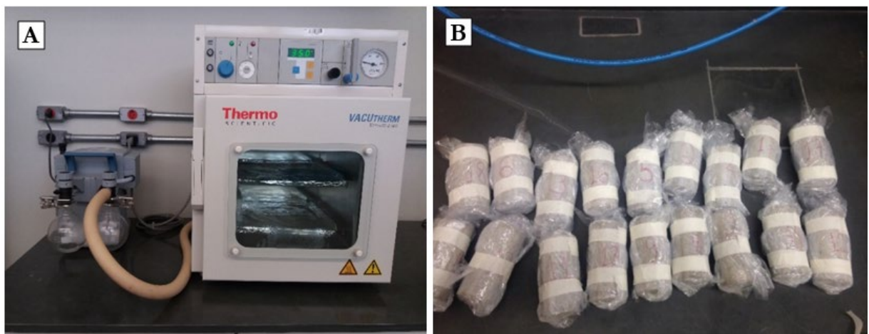
Figure 1. Stages of the precondition adopted: 1 a Stage - vacuum oven (A) and 2 a Stage – Samples packaged in a plastic film (B).
