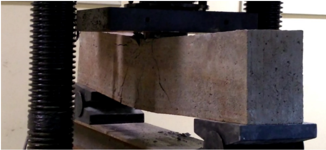
Figure 10. Rupture of beam VA57.
