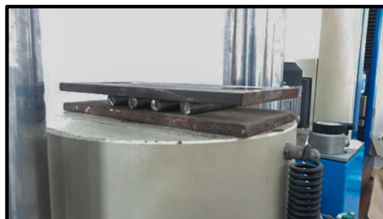
Figure 6. Set of steel plates and rollers for the direct shear test of push-off specimens [15].
