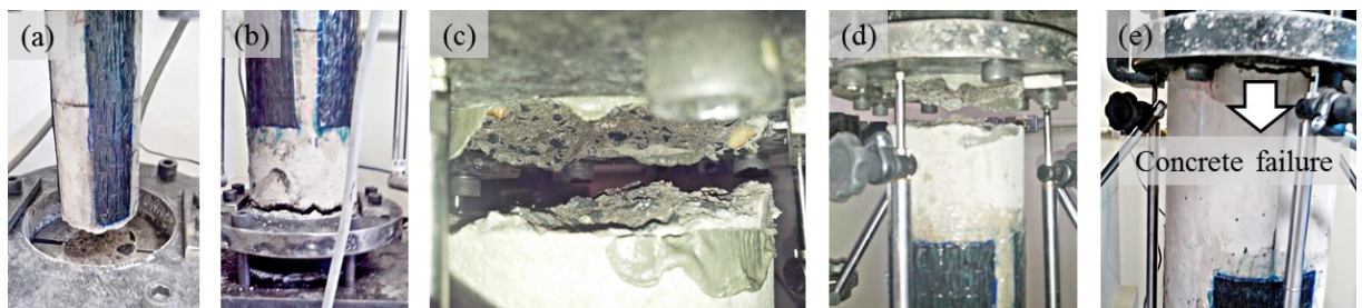
Figure 8. Experiments with concrete failure: a) FRP geometry G02 and 50 mm × 100 mm specimens; b) FRP geometry G05 and 100 mm × 200 mm specimens; c) FRP geometry G08 and 100 mm × 200 mm specimens; d) FRP geometry G10 and 100 mm × 200 mm specimens; e) FRP geometry G10 and 150 mm × 300 mm specimens.
