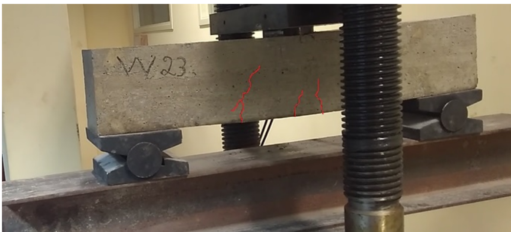
Figure 6. Cracks observed in the VV23 beam.
