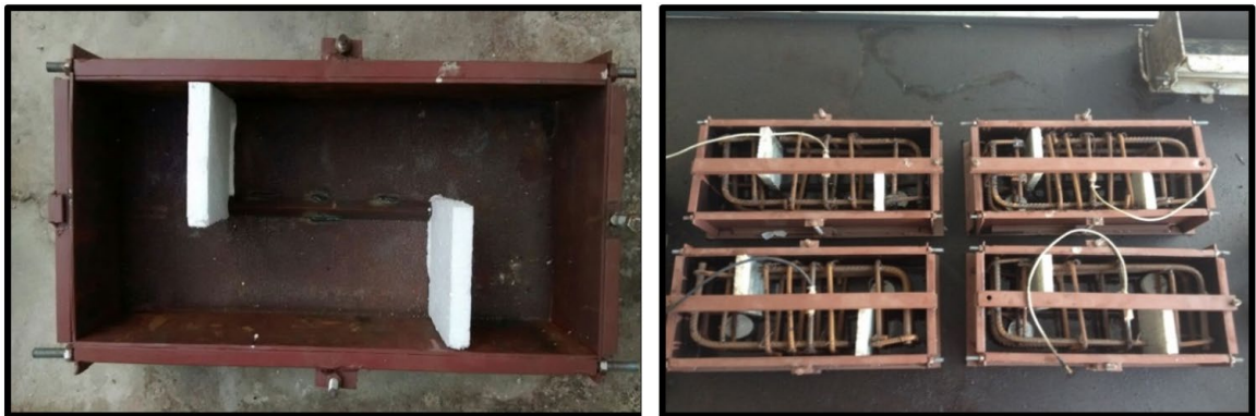
Figure 4. Metallic form for the production of push-off specimens [15].
