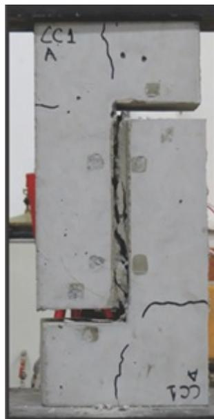
Figure 6. Rupture of specimen CC-A.
