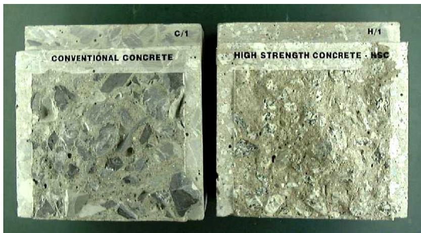
**Figure 6.** Conventional concrete (left) and high strength concrete (right) fractured faces.
