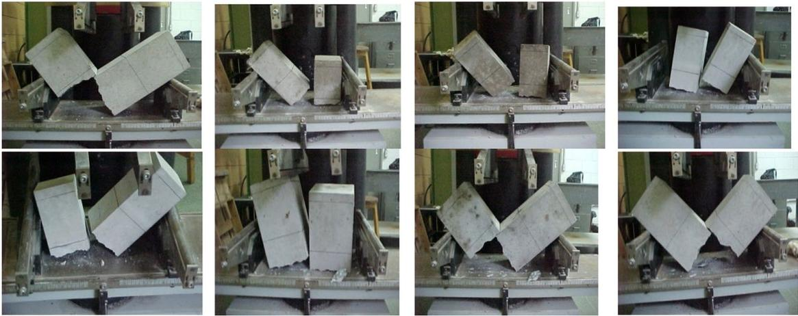
**Figure 12.** Fractured sections for the high strength concrete during fatigue tests.
