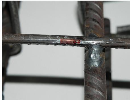
Figure 3. Steel bar instrumentation using strain gauge.
