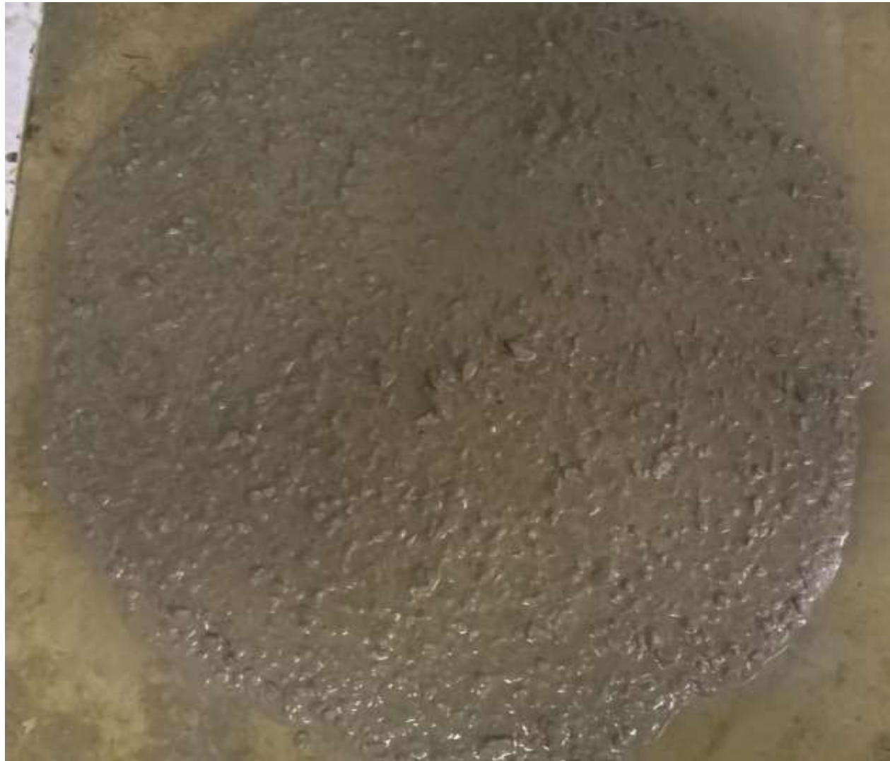
Concreto com aditivo mid-range
