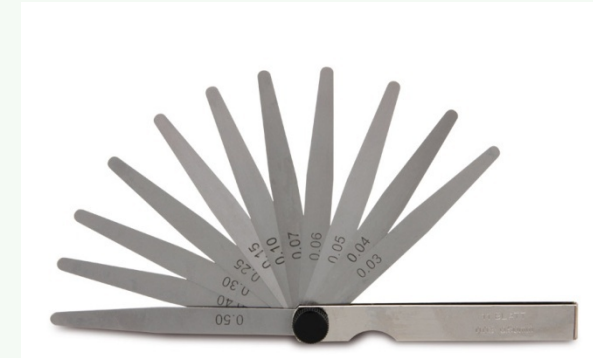
Crack width measurement
