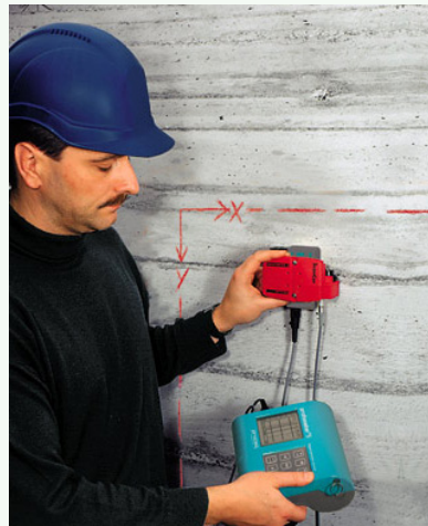
Concrete cover measurement
