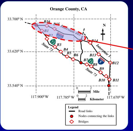
The seismic performance of the link (*LDI*) depends on the damage states of the bridges in the links.
