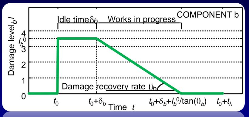
$\theta_{\rm b}$  cannot be higher than an upper limit (maximum recovery speed 80°). Moreover  $\theta_{\rm b}$  is never convenient below a lower limit (30°).
