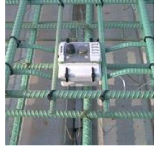
Embedded Corrosion Instrument – ECI
