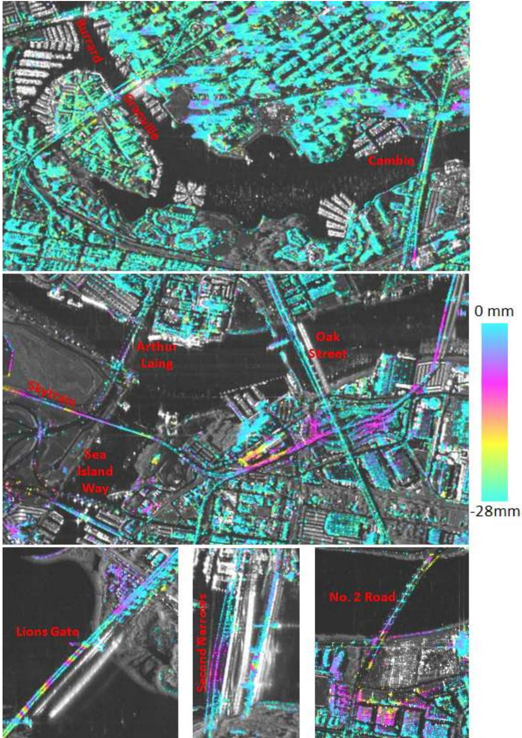
Figure 10 – Bridge Proximal Displacement Measurements of selected Vancouver bridges
