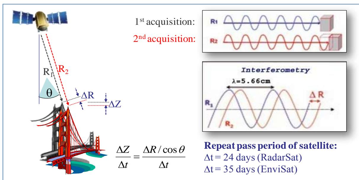
Figure 2 – SAR interferometry for remote monitoring of urban structures
