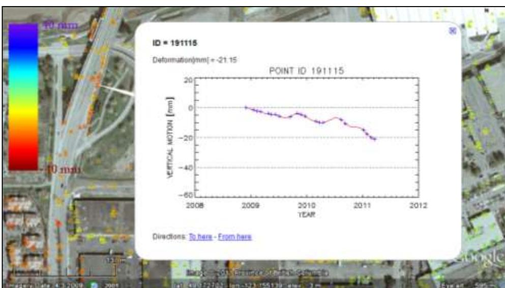
Figure 12 – Displacement over two years of a point target on a bridge approach slab
