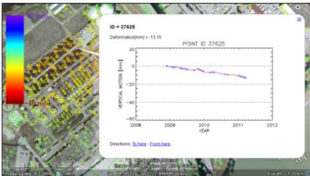
Figure 11 – Displacement over two years of a point target on a wastewater treatment plant
