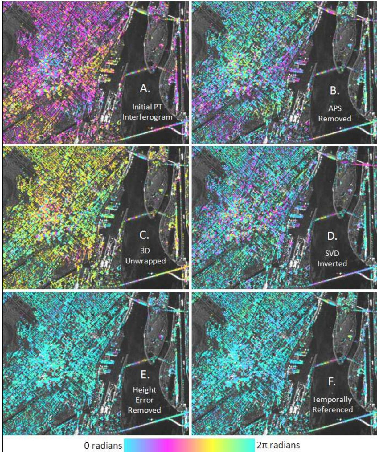
Figure 8 – Interferometric processing of a dataset over Montreal, QC representing signal phase change ( $2\pi = -28$  mm) from Jan 28, 2011 to March 17, 2011 and showing Jacques-Cartier br. (top); de la Concorde br. (middle); and Victoria br. (bottom)
