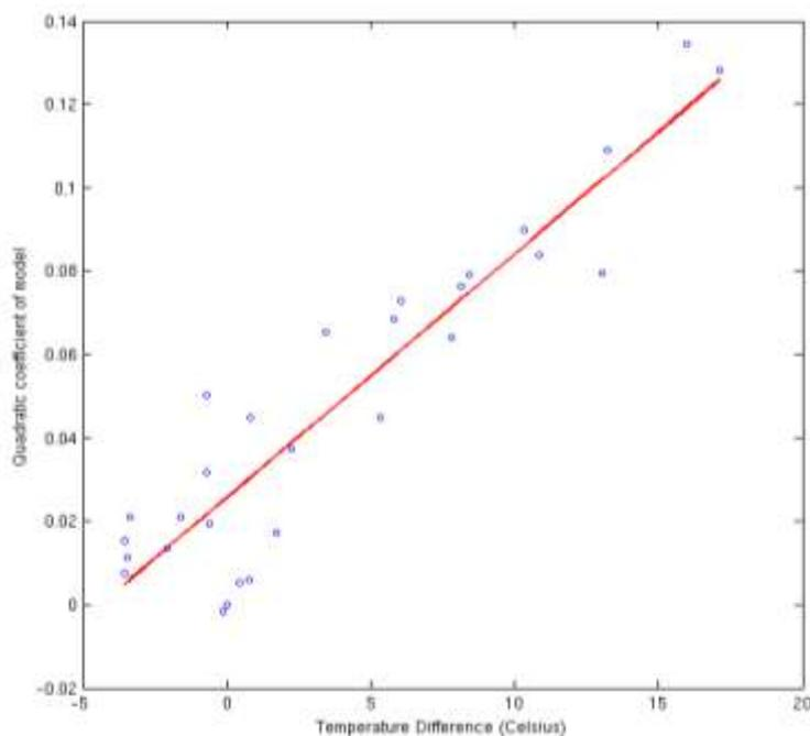
Figure 15 – Correlation between quadratic coefficients and temperature changes from the first interferogram (correlation coefficient is 0.93)
