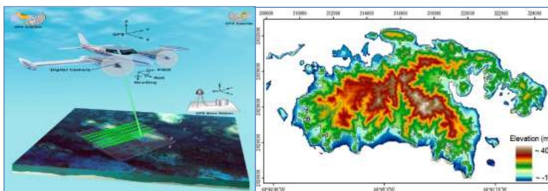
Figure 1 – LiDAR Process (left); USGS Elevation Results in St-Johns, U.S. Virgin Islands (right) (SCHREPPPEL and CIMITILE 2011)
