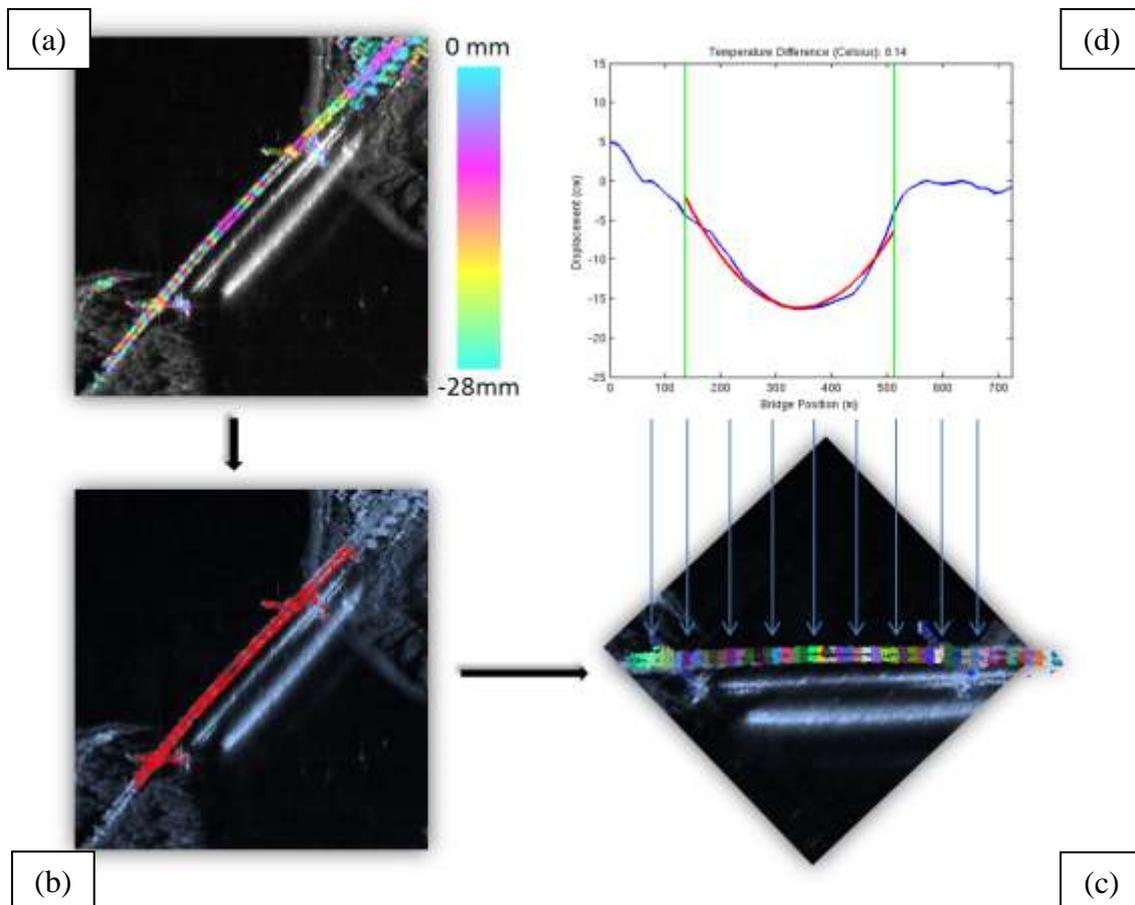
Figure 13 – Thermal deformation analysis of the Lions Gate Bridge
