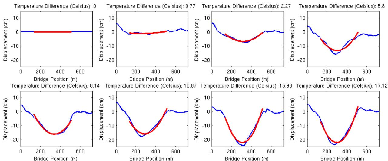
Figure 14 – InSAR-derived vertical displacement (blue) and quadratic fits (red) of the main span of the Lions Gate Bridge. Several profiles are shown with increasing temperature differences (left to right, top to bottom).
