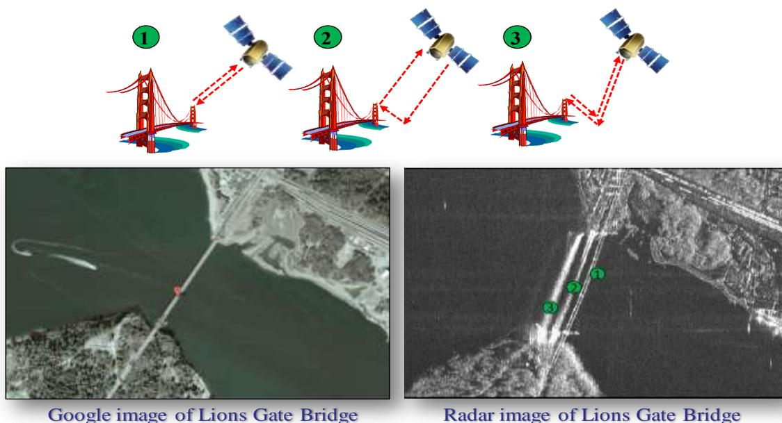
Figure 6 – Multi-bounce signal reflections in water near Lions Gate Bridge
