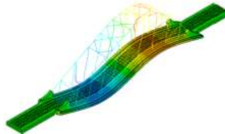
Mode 2 – f = 4.06 Hz Vertical bending
