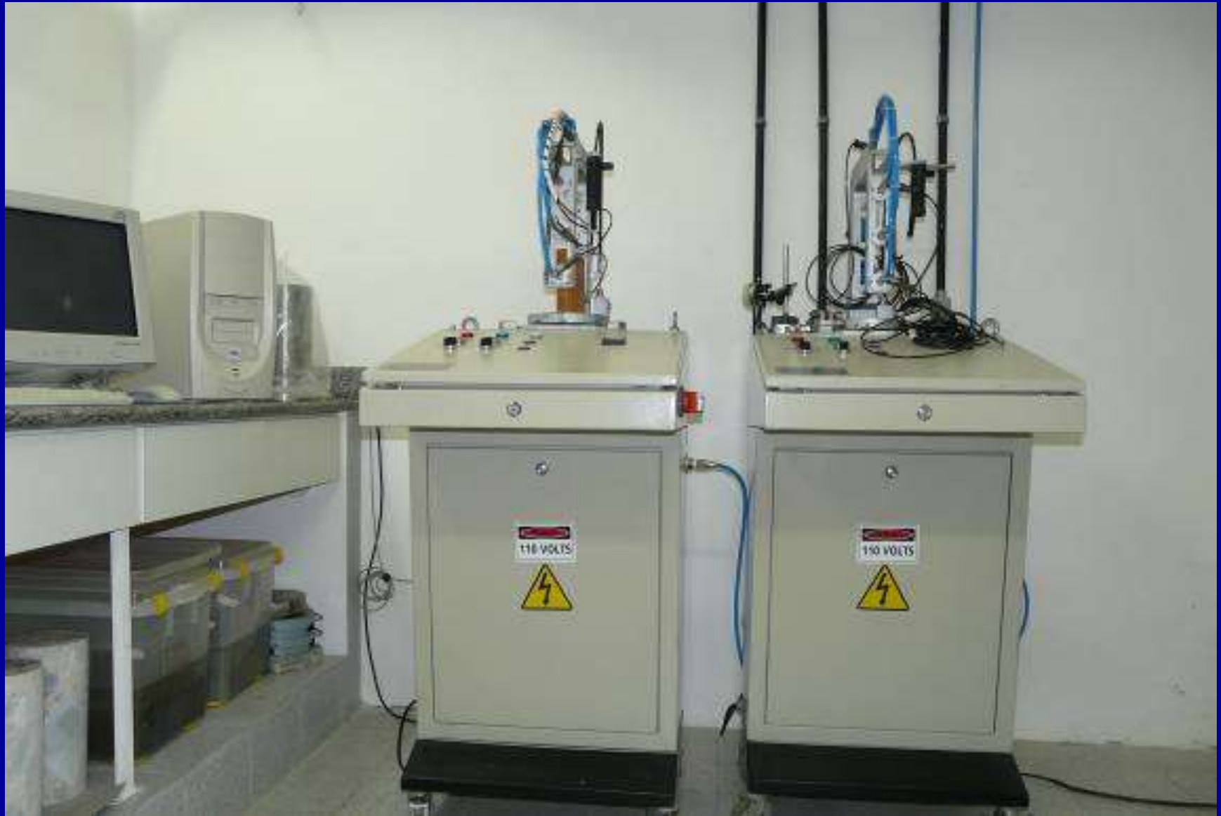
Robots (RMDV1 e RMDV2) for measuring volumetric delayed strains
