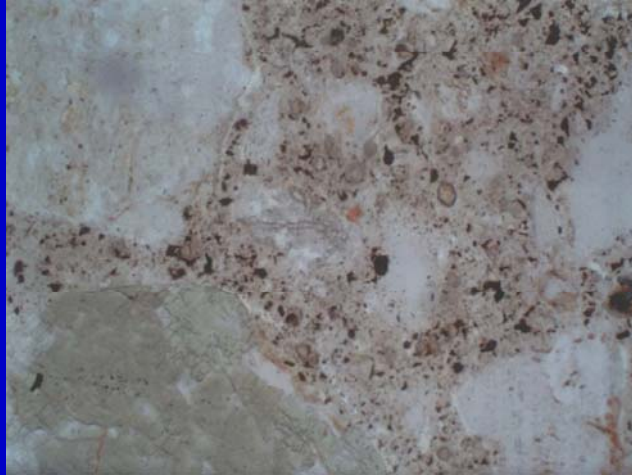
Photomicrograph of a thin section of HVFA concrete
