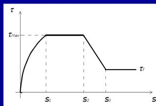
The reinforcement reaction and half the crack opening are given, respectively, by the integration of the bond stresses and the relative slips along the transfer length.
