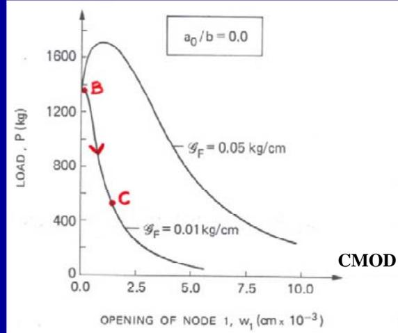
With a CMOD-controlled loading process, it is possible to follow the virtual softening branch BC.
