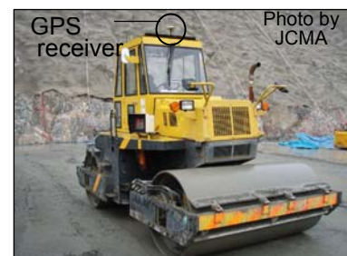
Photo 29- Vibratory roller SD451 with IT, Kasegawa dam
