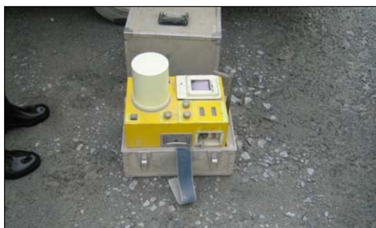
Photo 25- Concrete density measuring by RI meter
