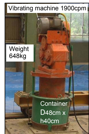
Photo 11- VC test with a large-size container
