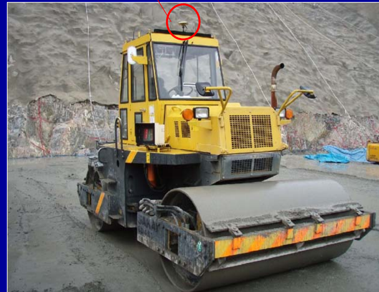
Vibratory roller SD451 with IT, Kasegawa dam
