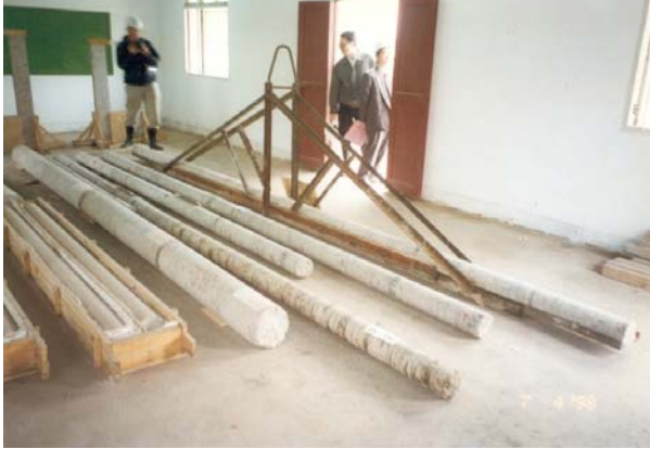
Photo 8 - Left, lengths of core up to 5m long from Jiangya Dam, right, 15.1m from Longtan Dam where horizontal lifts were placed within a retarded initial set time
